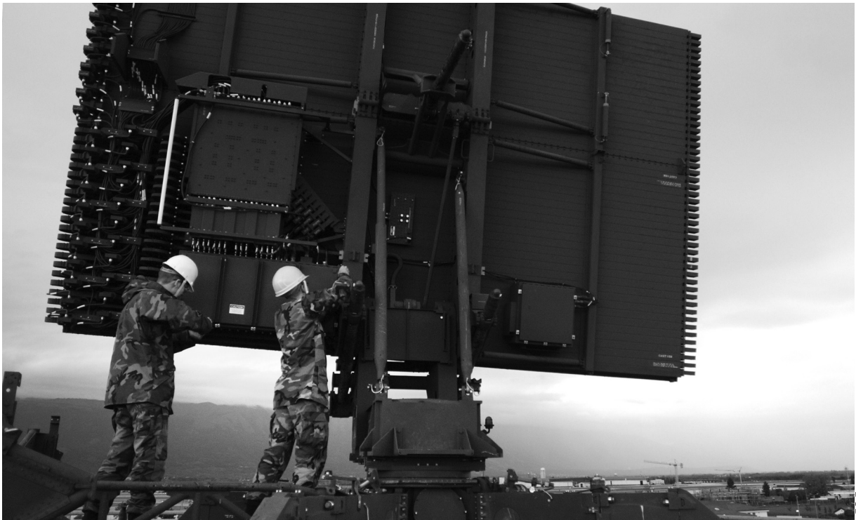
The TPS 75 Air Surveillance Radar System at Aviano Air Base, Italy, 5 October 2005.
