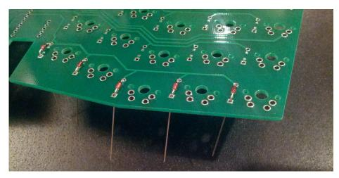
Once each set of diodes is soldered, trim the diode legs with wire cutters. Grip the diode leg as you trim it to keep it from flying across the room. Keep the diode legs; they will be needed in the next step. Repeat until each diode position is filled.
