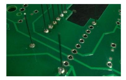
Fit the controller over the legs you've attached so far. Solder the four corner pins already connected to the PCB into the corners of the controller. (The bottom left corner is unused; the pin above it is used instead.) Try to ensure the controller is as close to the PCB as possible and not at an angle. Then solder the other left-side diode legs into the controller as well. Trim them all with your wire cutters when they are secure.
