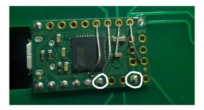
Before you go on, take the time to double-check the solder joints on the controller. The solder should fill the hole completely without spilling over to adjacent holes. Also check that all the diodes are facing the correct direction with the black band pointing to the bottom of the board.
