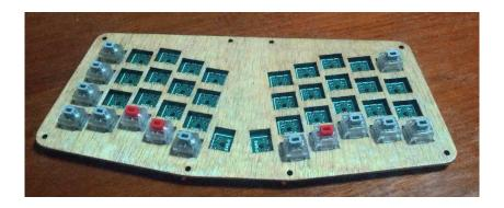
Next fill in the rest of the bottom row (SW1:3 through SW10:3) and the leftmost column (SW0:1 and SW0:2). If your kit has red linear switches which do not have any tactile bump, you can choose to use these for the modifier keys (shift, ctrl, alt, etc) or to leave the modifiers using the same switches as the rest of the board.<sup>8</sup> The modifiers on the bottom row are SW2:3, SW3:3, and SW8:3.
