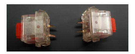
Connecting the center two rotated thumb keys (SW5:0 and SW6:0) in kits with Matias switches requires a little bit of tweaking. (Cherry switches do not need this step.) The holes for the pins are not aligned quite under where the pins protrude. A little twisting will allow them to go in nicely. Note that the two switches must be twisted in opposite directions since they are oriented facing
