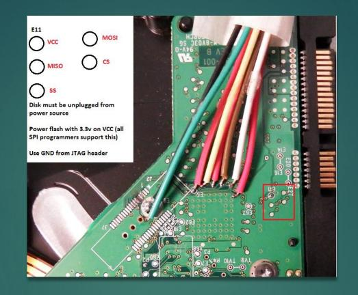
In my case the connection point for the SPI programmer is a cluster of 5 metal contact points on the bottom of the drive.
