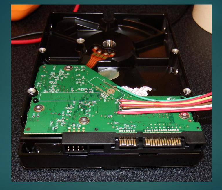
JTAG and SPI wires are soldered directly to the PCB
