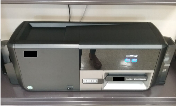
Fig. 18: The HID Fargo DTC5500LMX automated encoder our university uses to produce ID cards. We have obscured labels to maintain anonymization.
