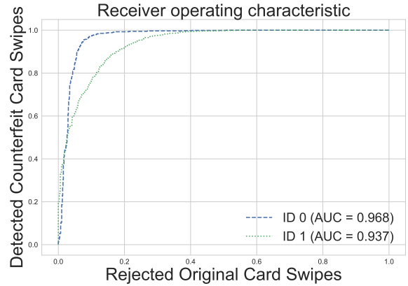
Fig. 12: The ROC curve for low-quality cards shows good detection even in non-optimal conditions.
