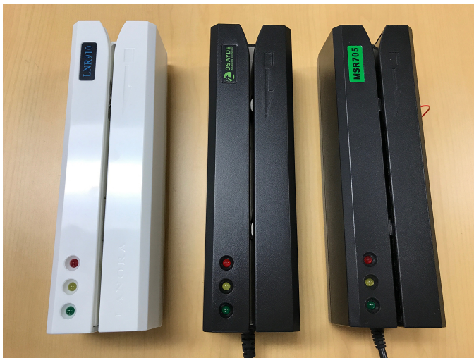
Fig. 5: The three manual card encoders we examined (from left to right): the Lanora LNR910, Osayde MSR605U, and the Misiri MSR750. Despite being sold under different brands and vendors, these devices are functionally identical.
