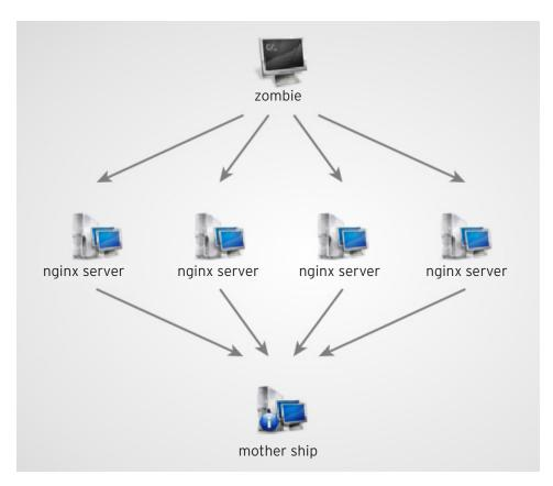
FIGURE 10: Typical C&C infrastructure layout of the Asprox botnet
