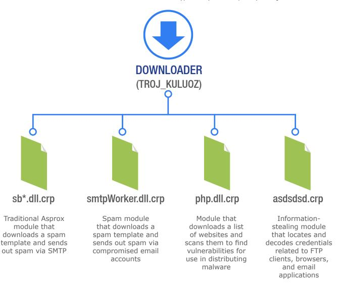
FIGURE 12: Asprox botnet components or modules
