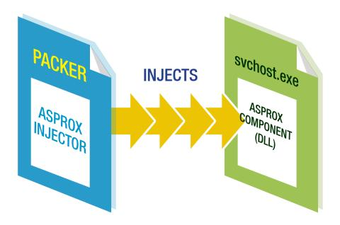
FIGURE 7: How the Asprox malware infects a computer
