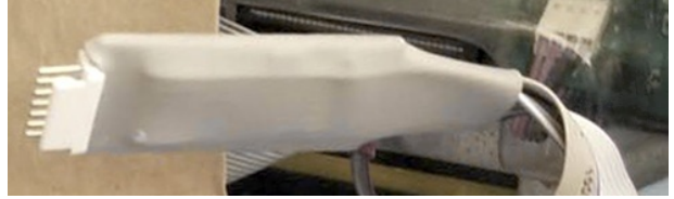
Figure 1: An internal Bluetooth-based skimmer wrapped in grey tubing to blend in with the cabling inside the fuel pump. This skimmer was detected by Bluetana in Tempe, AZ.
