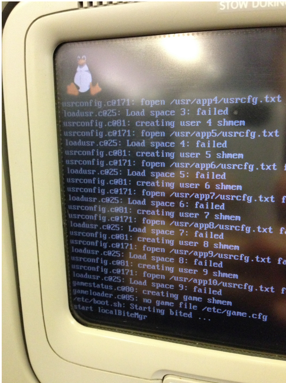
Figure 6: This airplane entertainment system running Linux crashed on my plane. While entertainment is not safety critical, imagine if flight control systems accidentally had a pathway to the entertainment software. Automobiles used to separate entertainment systems from engine control. However, a programmer eventually mixed the two systems unwittingly, enabling hackers to take control of an automobile by infecting the entertainment system.
