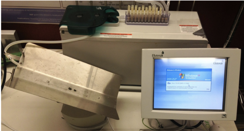
Figure 9: This is a pharmaceutical compounder from my lab at the University of Michigan. Hospitals use this device to mix custom, liquid drugs for IV delivery. FDA received a complaint that this model of compounder was infected with a virus. We found the machine to be running Windows XP, an insecure operating system. It was trivial to infect. A former employee of the company further explained that when the compounder was brought in for repair, the malware was accidentally spread to other compounders under repair.
